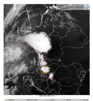
Fig. 18. RDT product derived from METEOSAT/SEVIRI satellite data with the EUMETSAT NWC SAF Geo package, 11 August 2017, 19:00. The color of the contour marks the convection phases: yellow = triggering, orange = triggering from split, red = growing, purple = maturity and blue = decaying.
